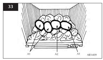
9.16 Place the remaining two pebbles identified as shown in diagram 34.
